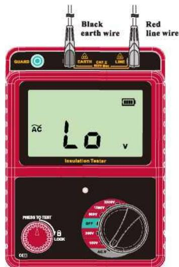
3、 After the full LCD display one sec, the LCD shows as below, do not press TEST button, the unit have the auto AC detection function.
