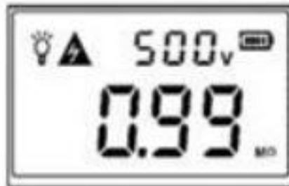
Until contrarotate and release the TEST switch to original position, the high voltage indicator and Alarm will turn off gradually, instrument on testing status, release the button the unit will auto discharge the voltage .Only disconnect the testing wire after the LCD Display 0v.
