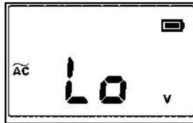
4、 Connect the red black wire or pin to the tested electrode the LCD shows the reading as below:
