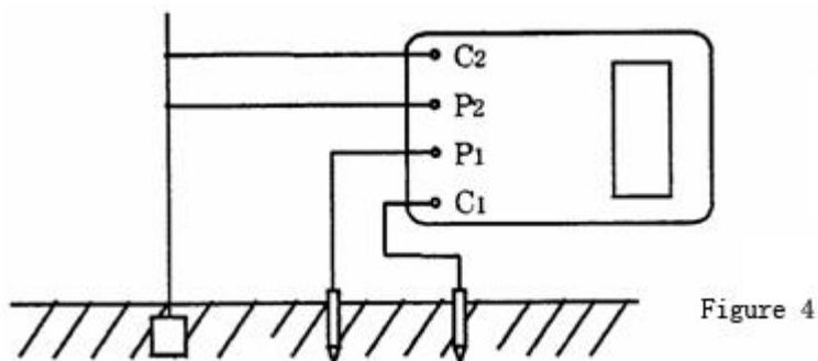
3. When measuring grounding resistance of large grounding grid, the wiring method is different from the general method, detailed wiring please refer the measurement requirement of current meter or voltmeter.
